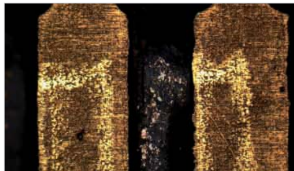
... as a result the contacts fell off the pads and caused contact interruptions.
